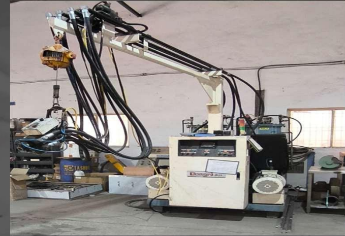
PU Foaming M/c For Refrigeration Products
